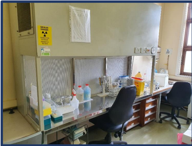
Image 2.1: Laminar flow cabinet in which all sterile procedures were performed regarding the Whole Blood Stimulation preparation and process.
