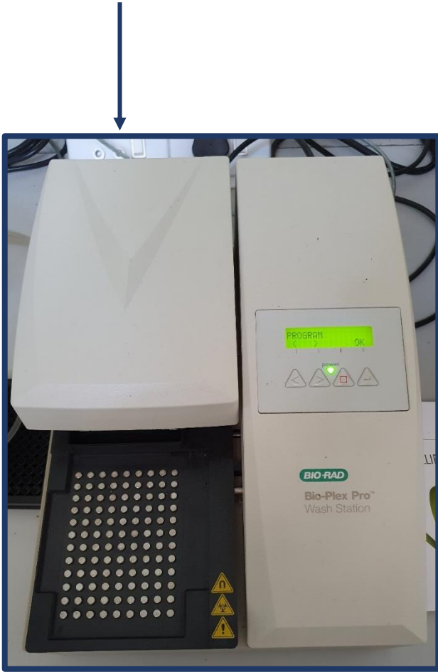
Image 2.10: Bio-Plex Pro Wash Station which was used for plate washing as part of the Immunoassay process.
