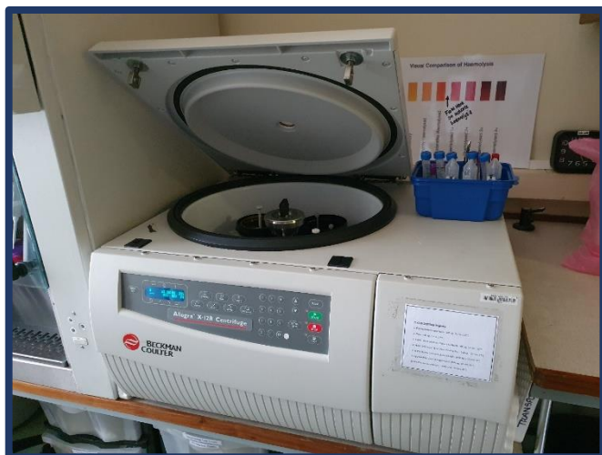
Image 2.4: Allegra X-12R centrifuge which was used to centrifuge the WBS samples after the incubation step had concluded.
