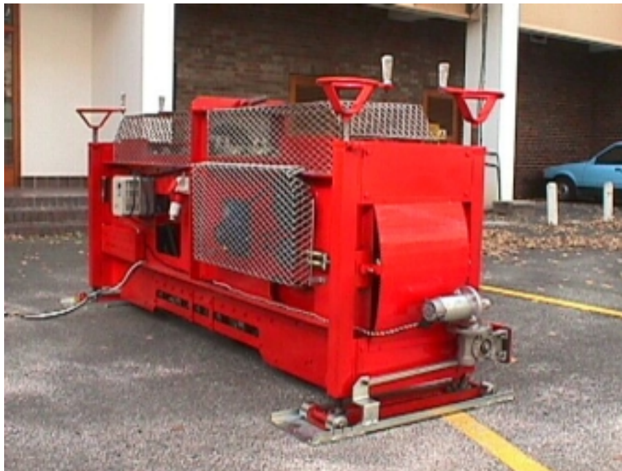
Figure 2. General Configuration of MMLS Mk3 APT device
