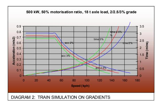
The analysis indicated that a 2.5% grade could be accommodated with 50% motorised axles and a power input of 500 kW for each motor.
