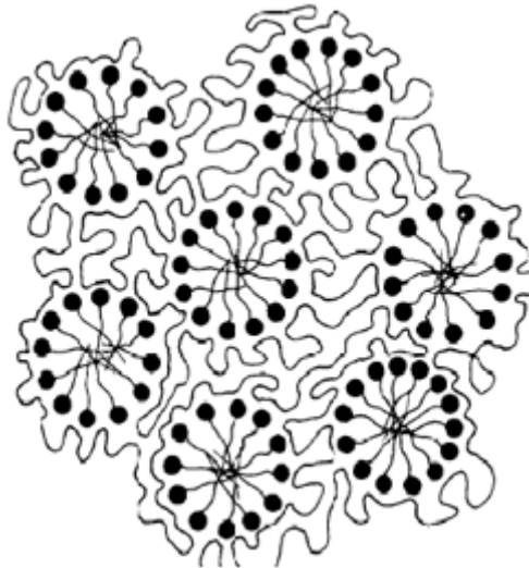
Figure 14. Schematic representation of polymer-micelle complexes topology in aqueous solution (Nagarajan, 1985)
