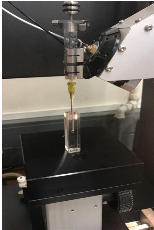
Figure 29. Water-oil surface tension measurement.
