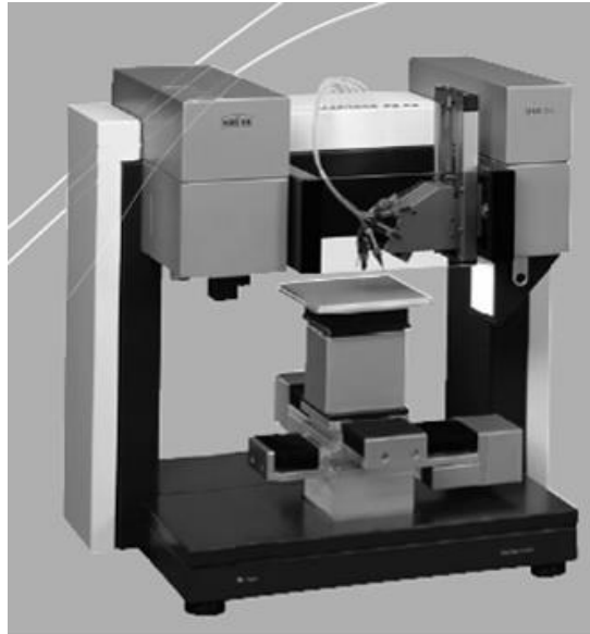
Figure 27. Drop shape analyser (KRUSS DSA 100 Tensiometer) used for determining surface tension.
