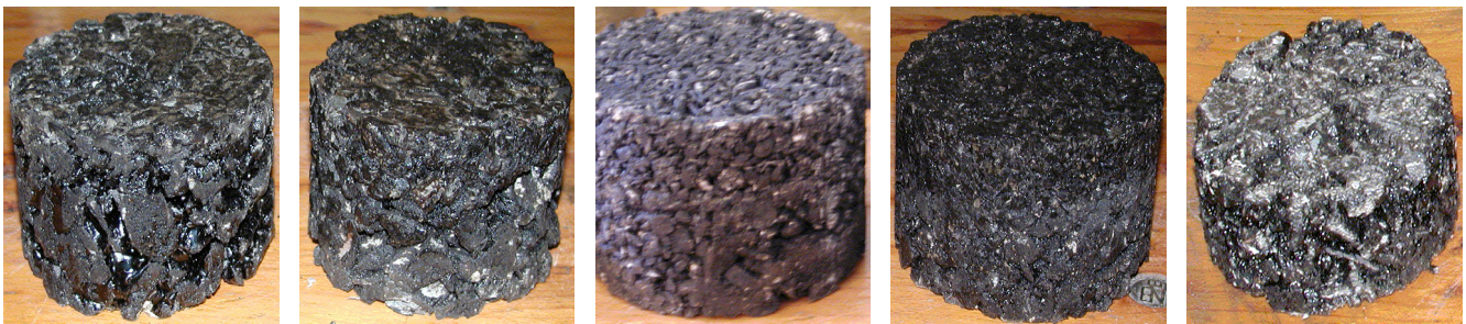
Figure A-1: Photographs of Marshall briquettes, from left to right, Fluisterfalt, Cityfalt, Superfine Twinlay and Conventional Porous Asphalt.
