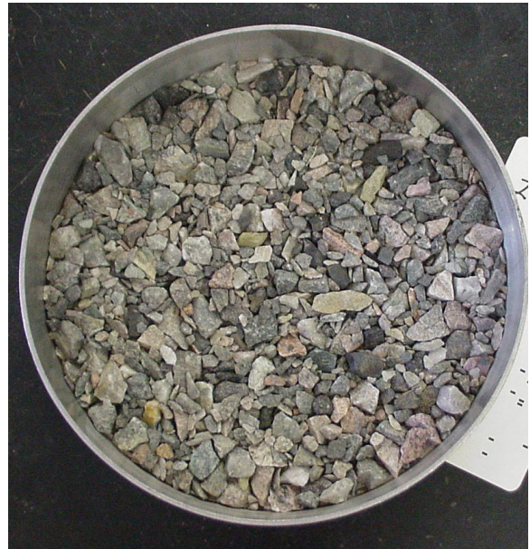
Figure 6: Stone application rate of small stone on top of large stone was 5\text{ kg}/\text{m}^3 (i.e. 259\text{ m}^2/\text{m}^3 ). Example of a "one-and-a-third seal".
