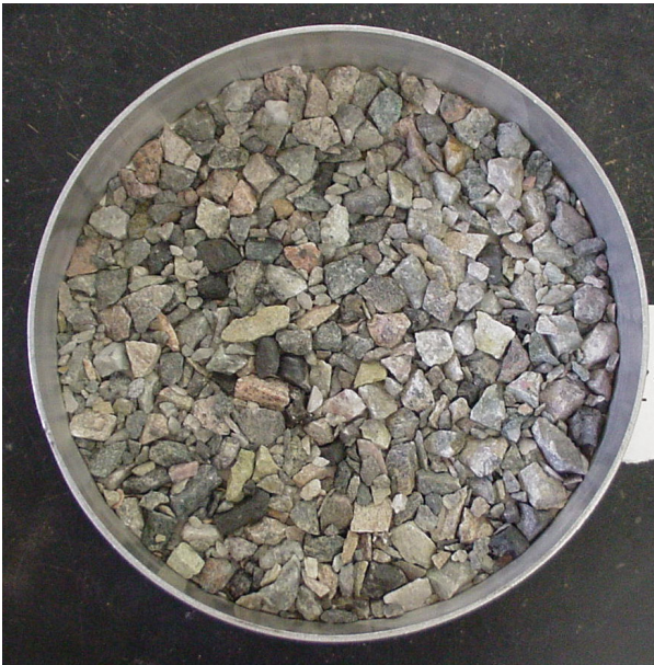
Figure 5: Stone application of small stone on top of large stone 3\text{kg}/\text{m}^3 (i.e. 432\text{ m}^2/\text{m}^3 ). Example of a single layer choke seal.
