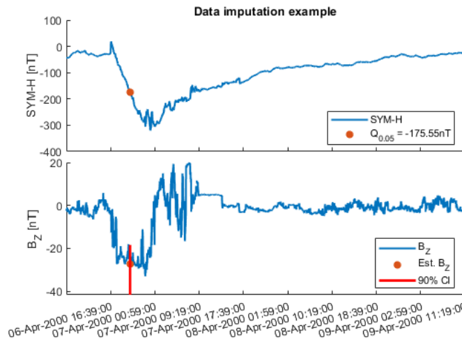
Figure 5.11: Utilising the SYM-H 95 th percentile distribution of B_Z (green curve in Figure 5.10), an estimate for B_Z is calculated and the 90% confidence interval is given.
