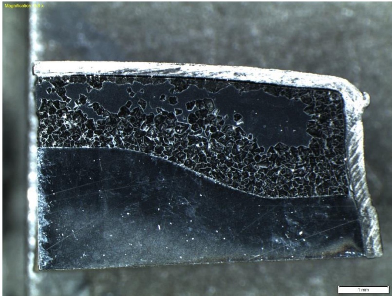
Figure 5.10: Optical image of the 0.5 \mu\text{m} sintered PCD doped with 3wt% \text{Cr}_3\text{C}_2
