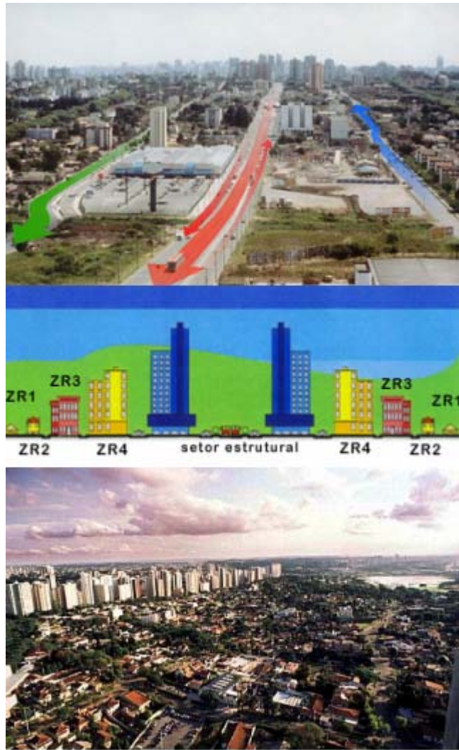
Figure 2. Corridor development concept: Bus-way and one-way street system.
