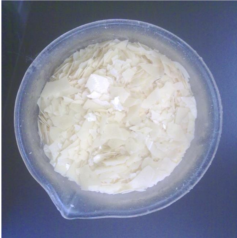
Figure B 4. Flakes of carnauba wax before being decanted and melted in Teflon sample moulds.
