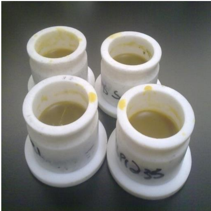
Figure B 5. Coal samples set in carnauba wax in labelled Teflon moulds.
