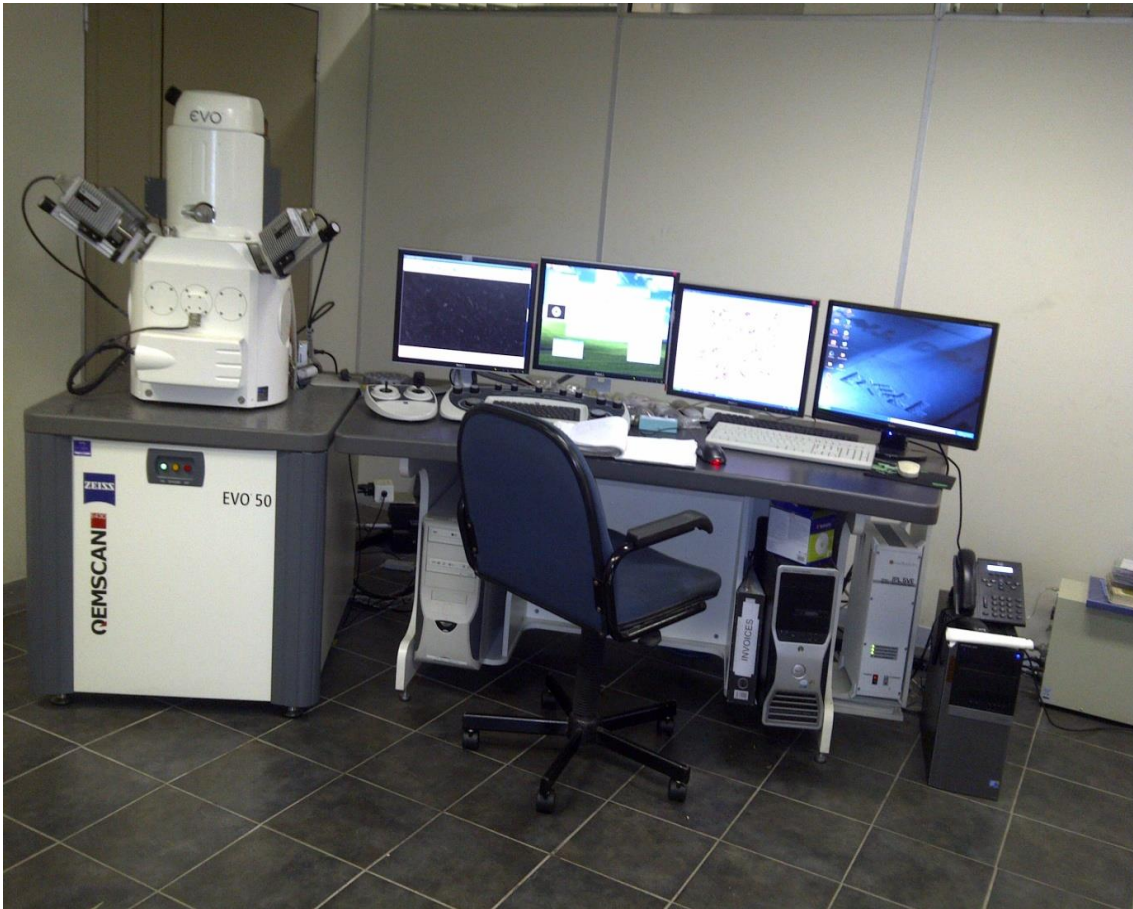
Figure 1. QEMSCAN comprising Zeiss EVO 50 SEM with four silicon drifted detectors based at ESKOM Research and Innovation Centre.
