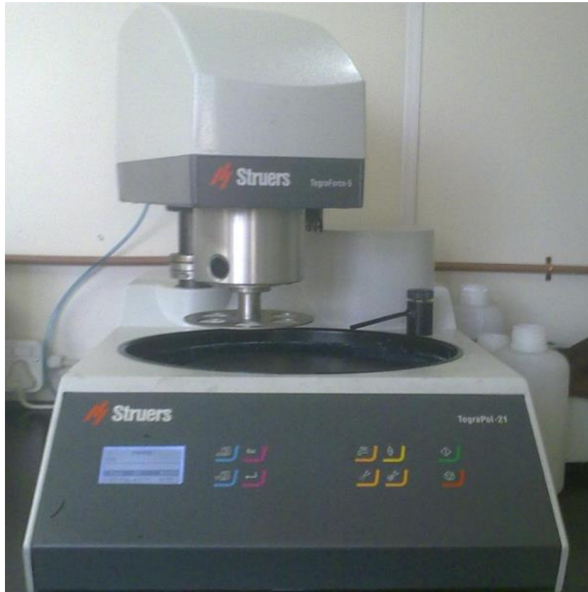
Figure B 6. Struers TegraPol-21 polishing instrument used to polish carnauba and epoxy blocks.
