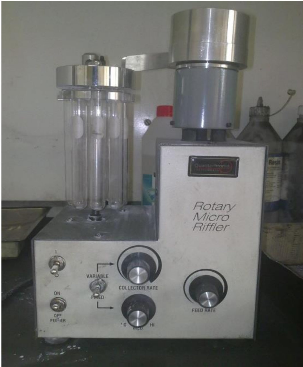
Figure B 3. Rotary micro riffler (Quantachrome Instruments) that splits the coal sample into representative samples.
