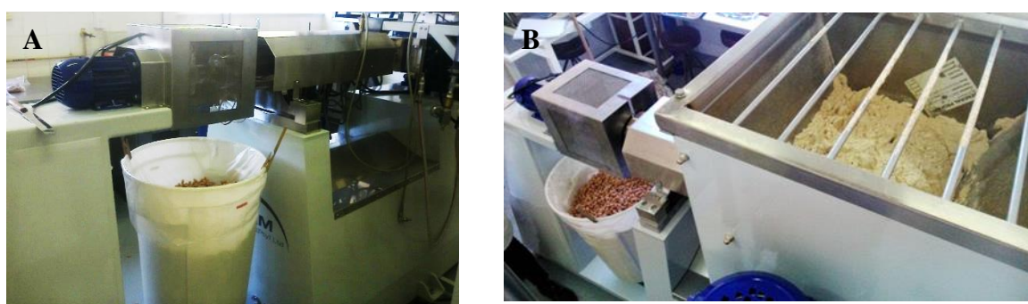
Figure 4.2.3 Extrusion cooker in process with the die end on the left of images
