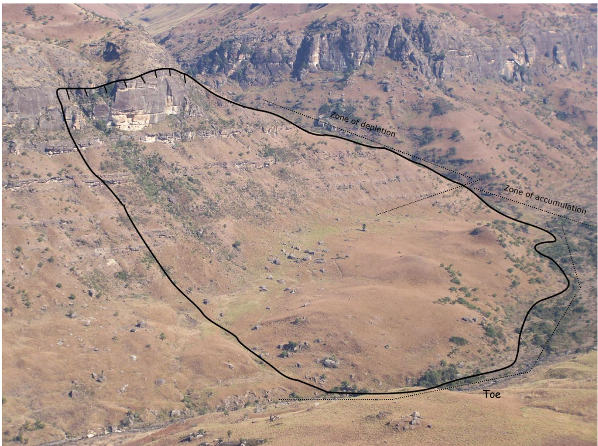
Figure 5.42: Aerial view of the Cataract movement. Depicted on the photo is the accumulation and depletion zone.
