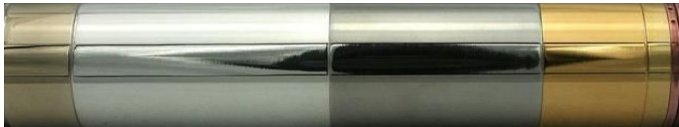
Figure 3.11. Surface Quality of Electroplated Metals (ArcelorMittal, 2006)
