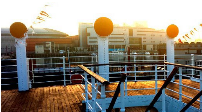
Figure 4.85. Lower First Class Lounge Dorade Vent on Flying Bridge Deck (McDonald, 2013)
