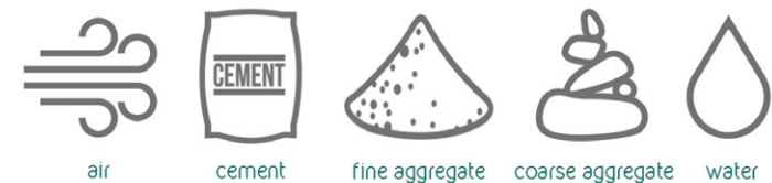
Figure 3.4. Components of Concrete (Author, 2016)
