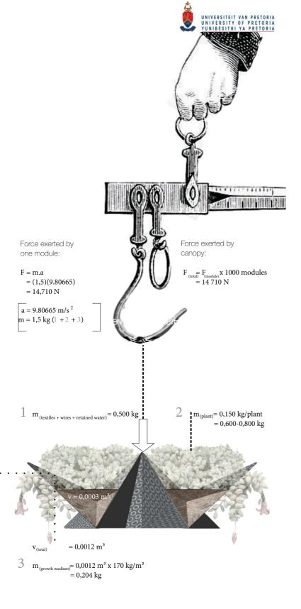
Figure 46: Forces exerted by canopy on supporting structure (Author 2016)
