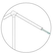
Scaffold steel hollow sections ac as conduits that carry irrigation pipes
