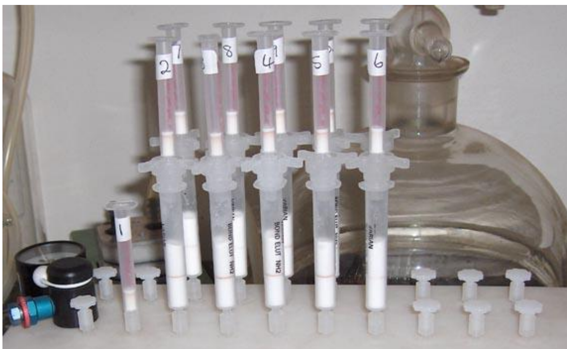
Figure 6.1. The second solid phase extraction (SPE) step showing the octadecyl bonded silica (C18) SPE cartridges connected on top of the pre-prepared aminopropyl unendcapped bonded silica (NH 2 ) SPE cartridges containing one gram Na 2 SO 4 , connected onto the extraction manifold.
