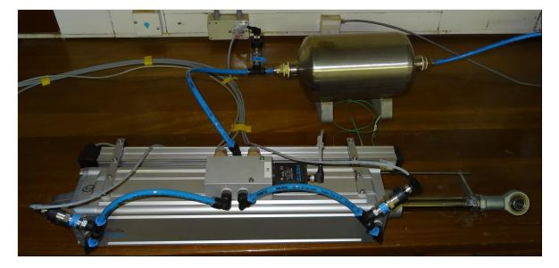
Figure 6.1: The Pneumatic Part of the Friction Identification Setup
