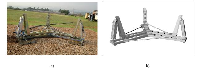
**Figure 2.3:** The SMS as a) Deployed During a Field Trial in Pretoria and b) as Presented by the Rhino3D<sup>®</sup> CAD Renderer
