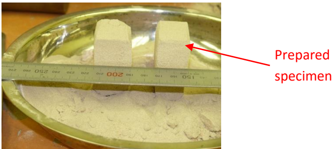
Figure 3.34b: Prepared SEM recovered tailings samples ready for desiccation
