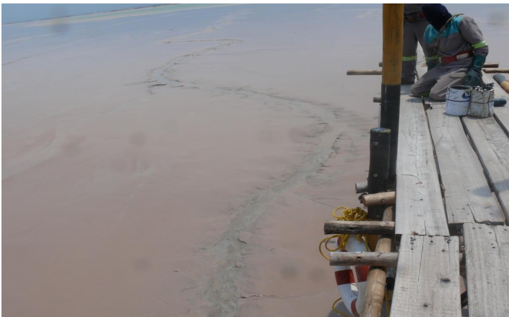
Figure 3.6a: Chemwes Dam 5 catwalk with deposited catwalk fines within reach for rope and bucket sampling. Channelling visible.
