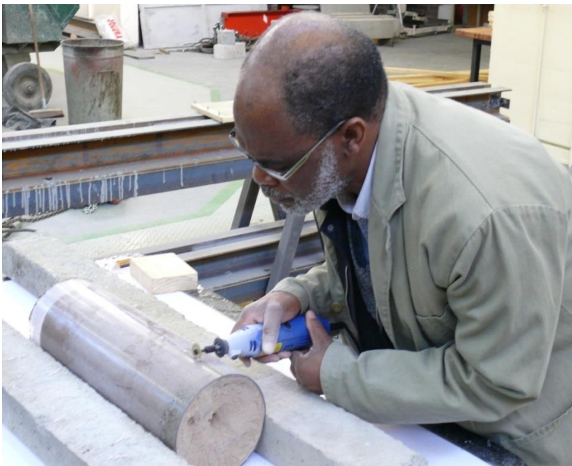
Figure 3.27b: Cutting open PVC tube to recover dried tailings
