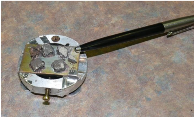
Figure 3.35b: Prepared SEM recovered tailings samples sputter coated with gold
