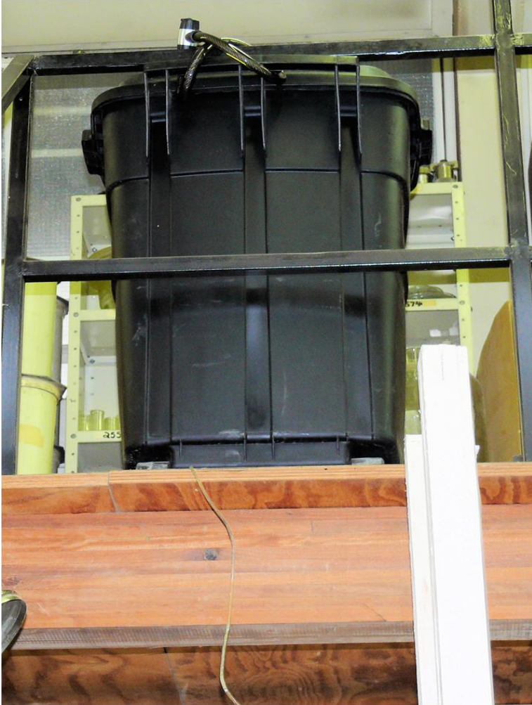
Figure 3.24a: Permeability 1000L water reservoir
