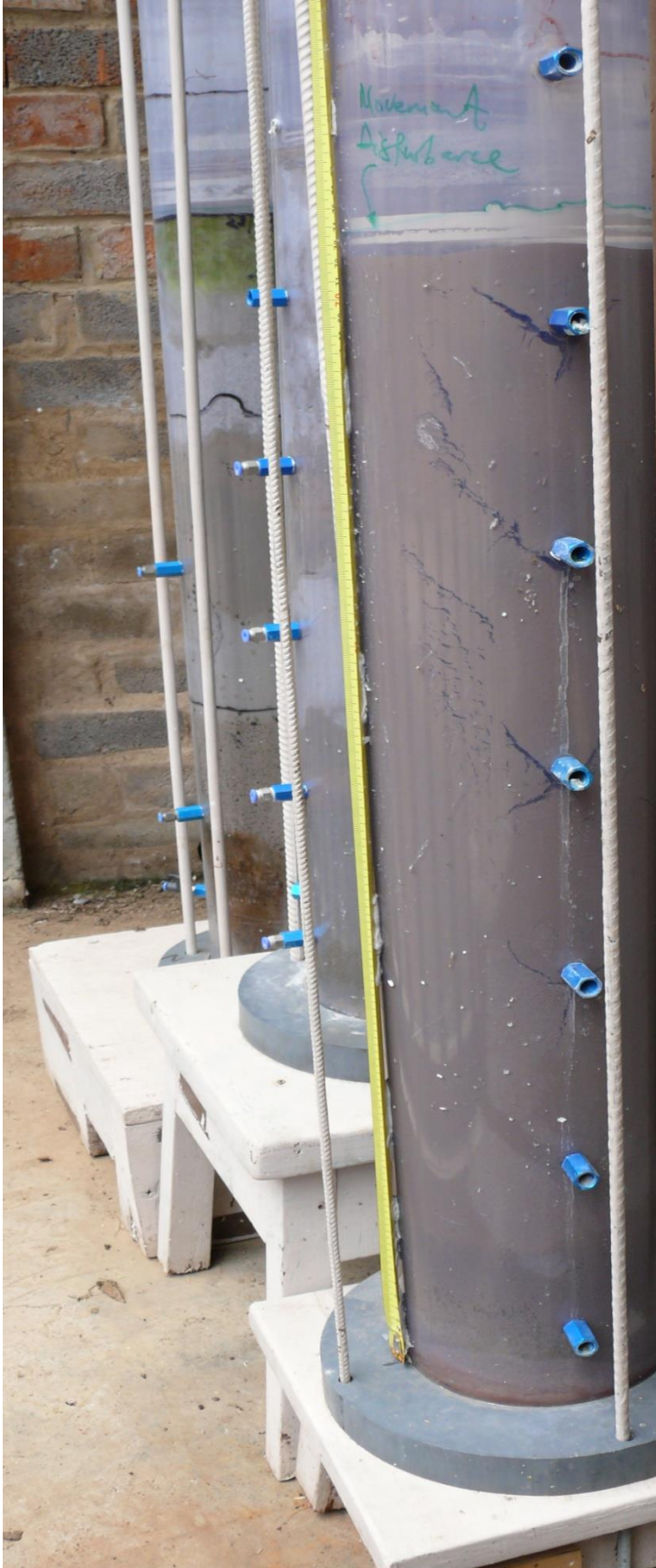
Figure 3.26: Experiments FDB, RoR20B and RoR10B settling columns tailings drying
