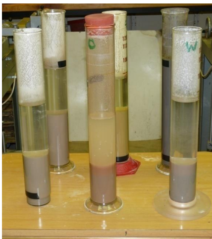
Figure 3.10b: 1000ml Cylinder sedimentation tests
