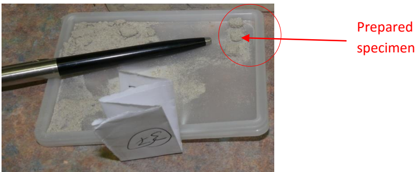
Figure 3.34c: Prepared SEM recovered tailings samples ready for desiccation
