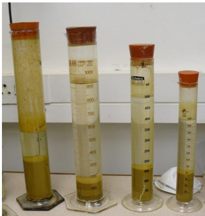
Figure 3.10a: Cylinder sedimentation tests different cylinder sizes
