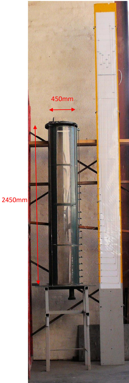
Figure A3: Large Settling Column apparatus
