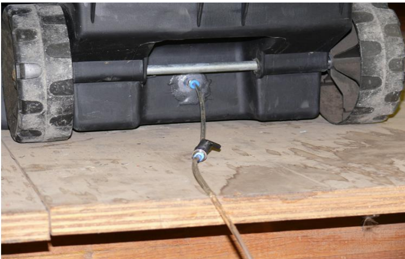
Figure 3.24b: Permeability water reservoir with water supply valve
