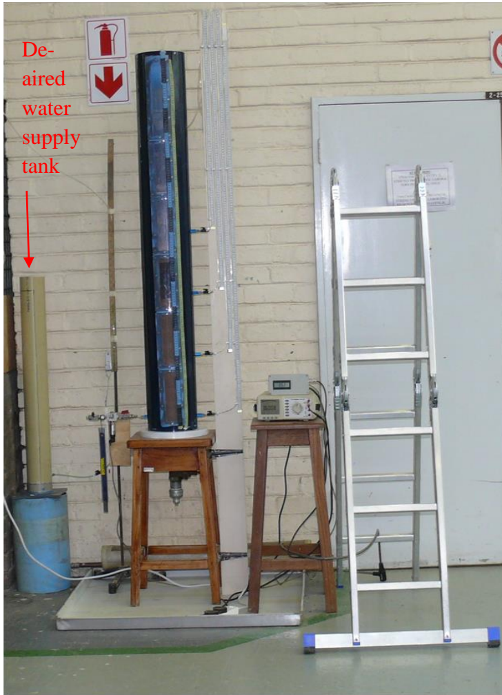
Figure 3.20: 190mm ID exploratory settling column (prior to modification into permanent settling column) and de-aired water supply tank
