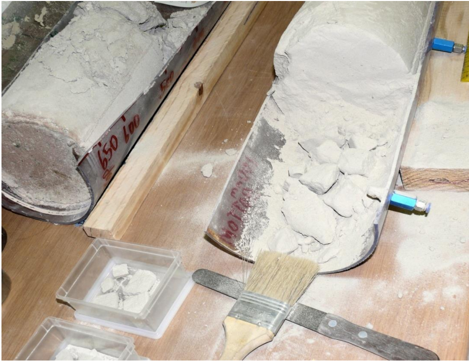
Figure 3.34a: SEM recovered tailings samples preparations
