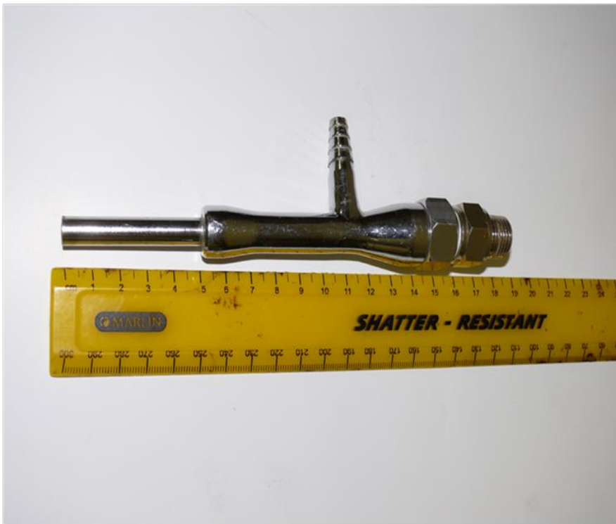
Figure 3.25b: Venturi meter for decanting water from settled tailings
