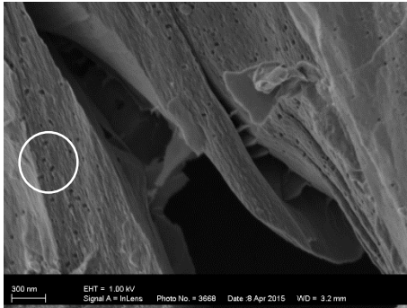
Figure 28 Cavities and cracks formed upon graphitisation (80 000x magnification)
