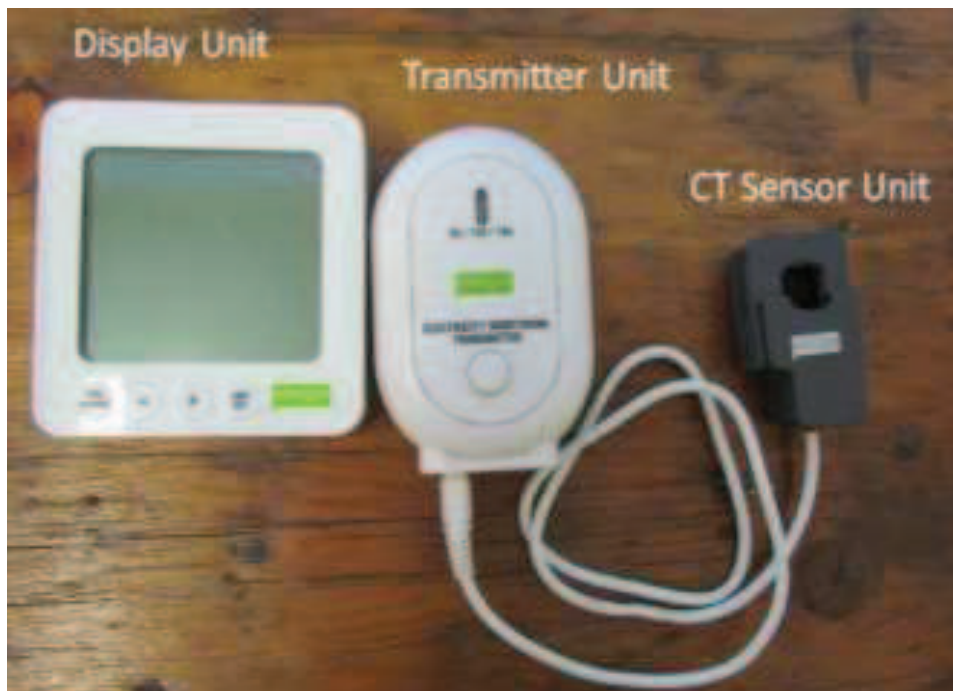
Figure 4.2: Efergy E2 classic energy monitor components
