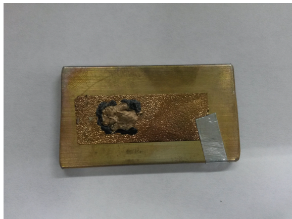
Figure 3.14: Segment of the lichen thallus, loaded onto an aluminium stub and coated twice with gold prior to SEM analysis
