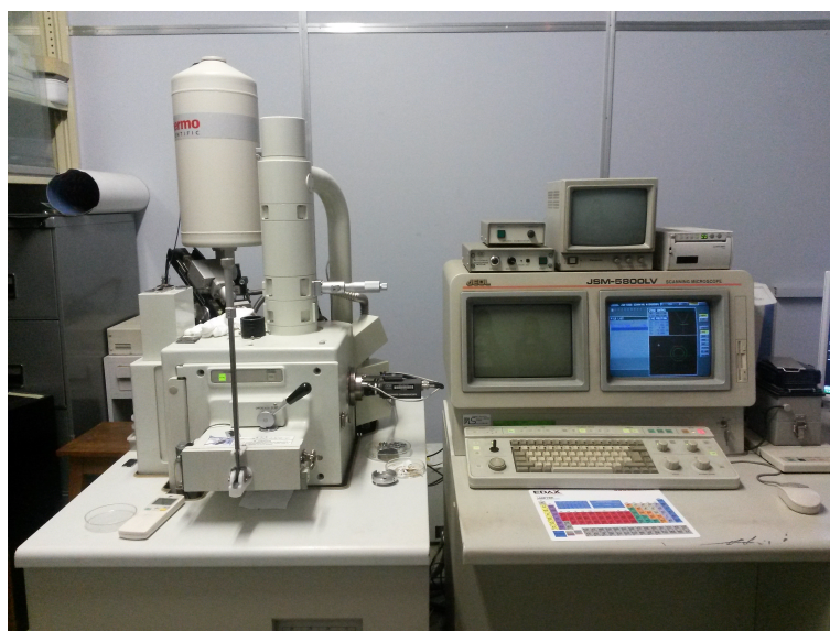
Figure 3.15: JOEL 5800LV SEM used for the analysis of the lichen segments
