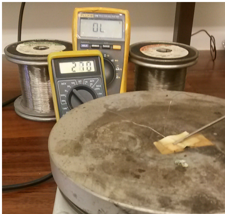
Figure 3.20: Combustion test on lichens using a hot plate and a thermocouple
