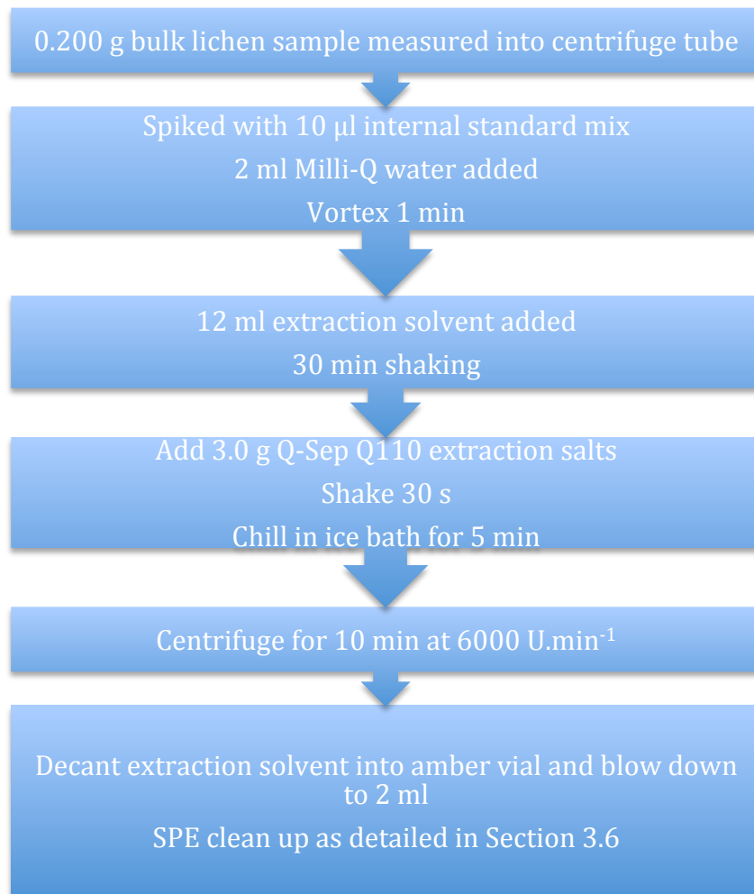
Figure 3.17: Schematic representation of the QuEChERS methodology used in this study to extract PAHs from lichens
