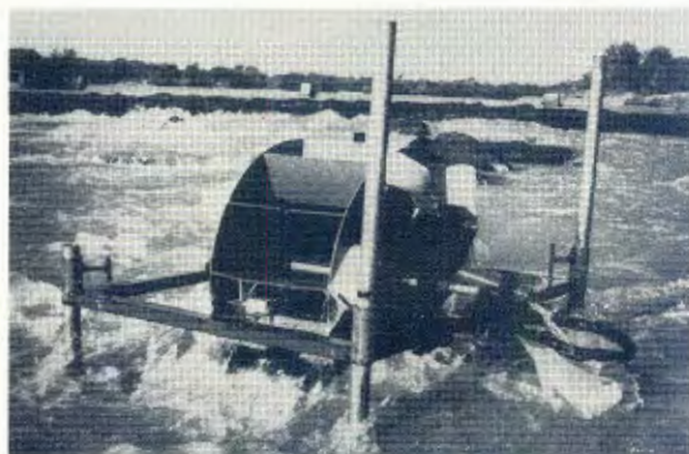
FIG. 1 Water-wheel drift sampler in the Orange River 100 m below the Marksdrift gauging weir
