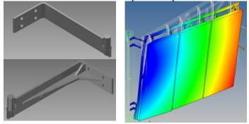
Figure 10: The first hinge designs warped badly
