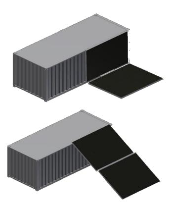
Figure 5: Side fold-out design allows all the panels to be packed away quickly but is still unwieldy to operate
