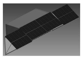
Figure 8: 'Book-style' - Struts are used to lift the solar panels to an optimal angle, based on the season
