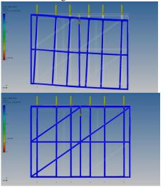
Figure 9: FEM analysis used to optimise the gate design
