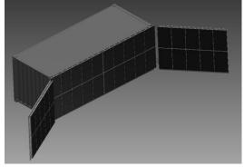
Figure 7: 'Book-style' - The security gates swing open revealing the solar panels
