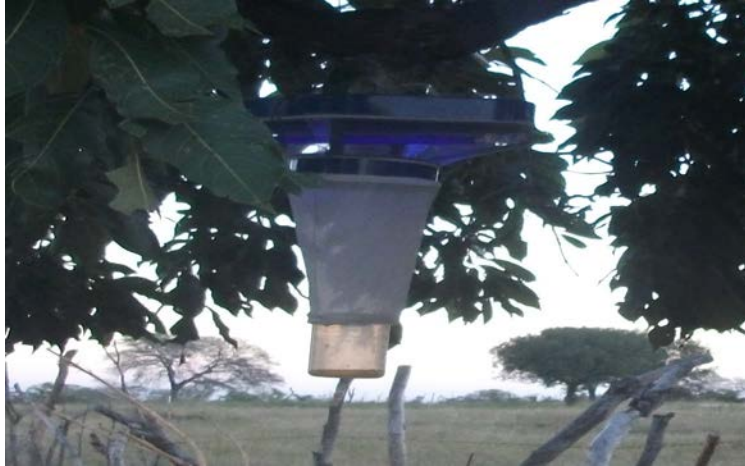
Figure 2.2: A 220V Onderstepoort light trap used for the collection of Culicoides species in Mnisi, Mpumalanga Province. © Jumari Steyn
