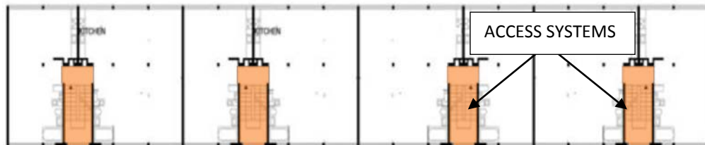
Figure 23: Access systems and circulation zones are strategically positioned and shared between apartments.
