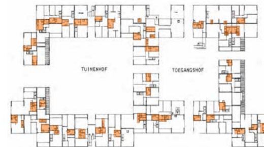
Figure 31: Services and wet services are determined by the users' at infill level. These are flexible and easily adaptable.
