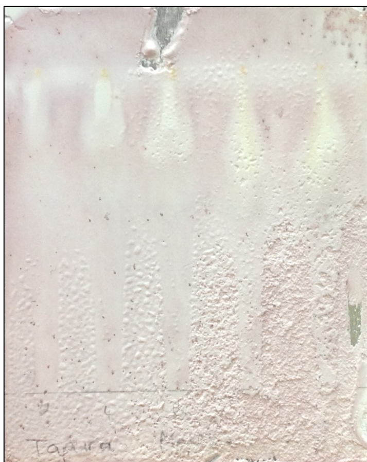
Figure 3.1: Bacterial inhibition (white spots) of E. faecalis by T. fischeri extract. The extract concentration increases from left to right. Inhibition is seen even at the lowest concentration. Mobile phase: 100 % MeOH.
