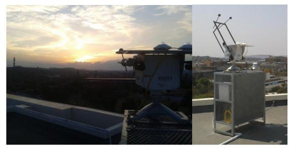
Figure 5.6 Solar measuring station to measure the DNI of the sun (SOLYS 2).
