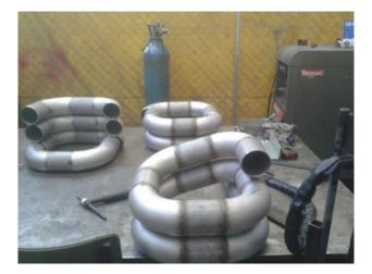
Figure 5.7 Manufacturing of the solar receiver.
