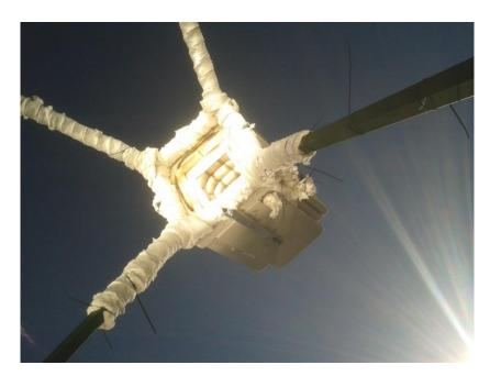
Figure 5.25 A bottom view of the solar receiver and its support structure during receiver testing with the blue sky in the background.
