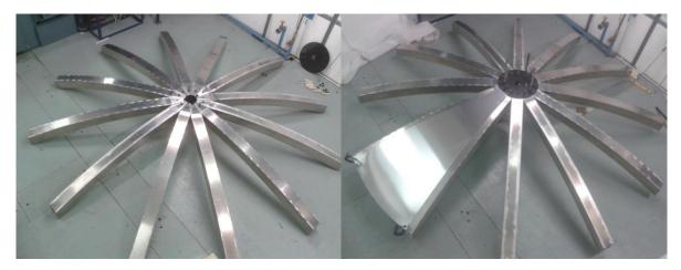
Figure 5.2 Assembly of the 4.8 m diameter parabolic solar dish in the laboratory (upside down).
