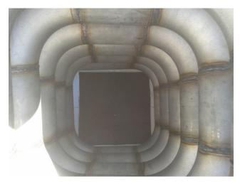
Figure 5.10 Top view of the solar receiver with the aperture shown at the bottom.
