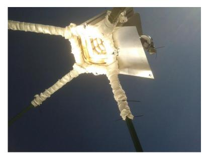
Figure 5.15 A view from the bottom: the illuminated receiver at the focal point of the dish during an experiment with the blue sky in the background.
