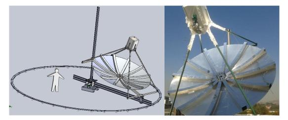
Figure 5.3 Test set-up as modelled in SolidWorks and as constructed showing the solar dish on the two-axis solar tracking system.
