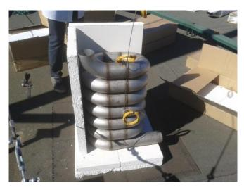
Figure 5.9 The solar receiver positioned on the bottom insulation before being installed on the receiver structure.
