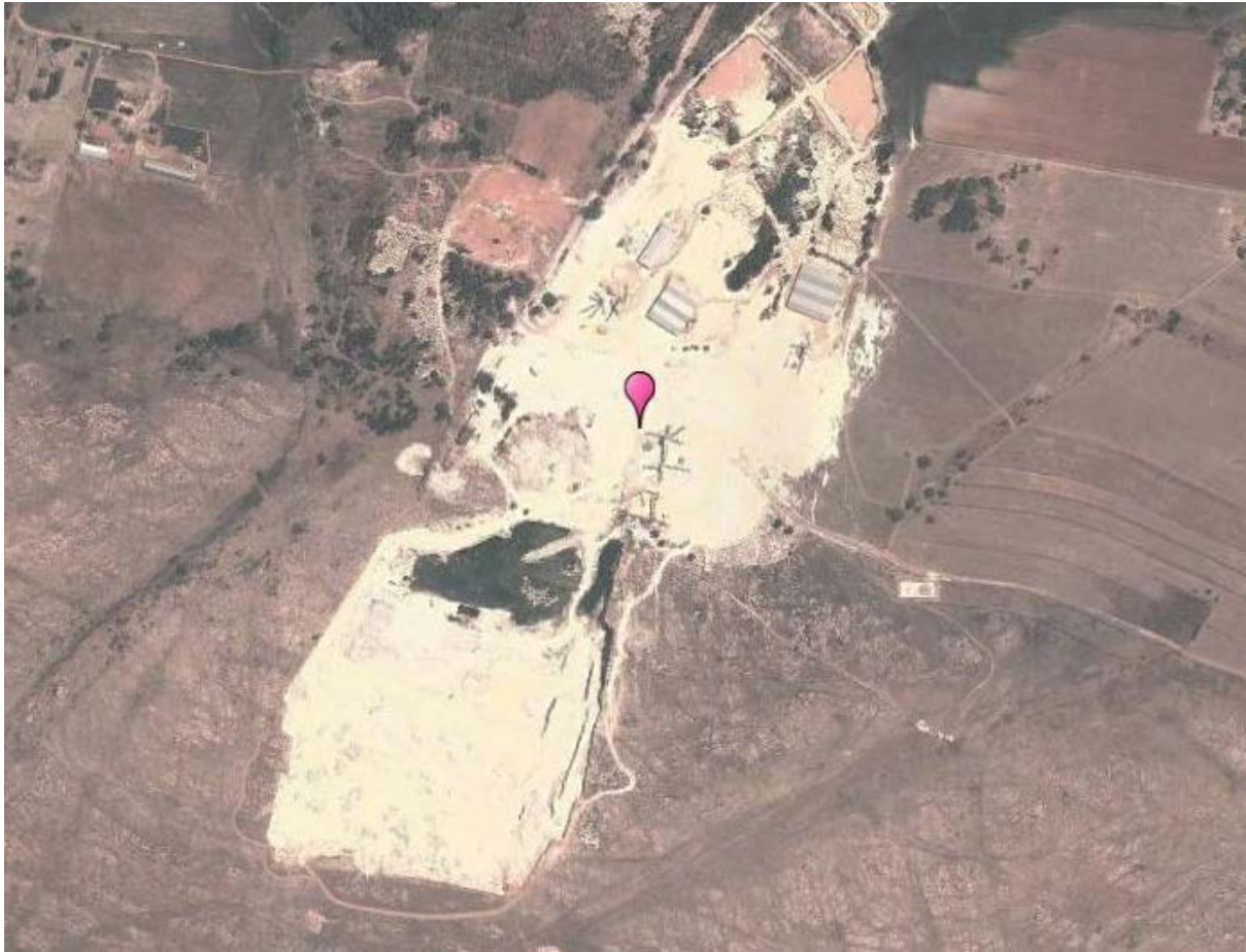
Figure 1.9: Google Earth map view of the Magaliesberg Formation study area (25°52'20.04"S, 28°39'28.75"E; pinkish bulb). Note the whitish colour of the freshly quarried sandstone which underlines the high mineralogical maturity (quartz >99%) of the sandstones.
