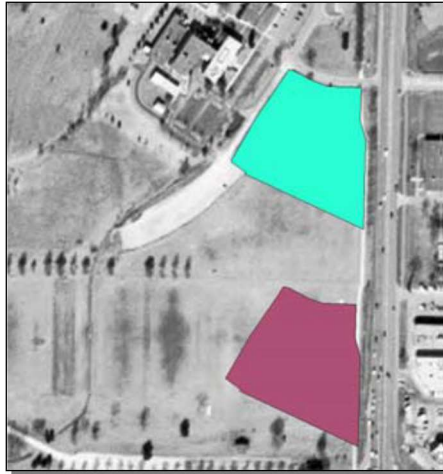
Figure 18 - Error caused by using the wrong datum (Egbert & Dunbar, 2007)
