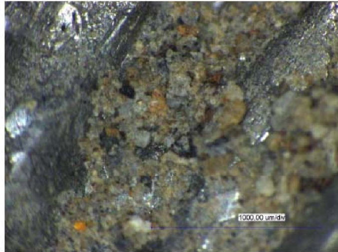
FIGURE 4: Two directional grooves and abrasive-embedding on the eroded areas of a liner in a slurry pump (x800).
