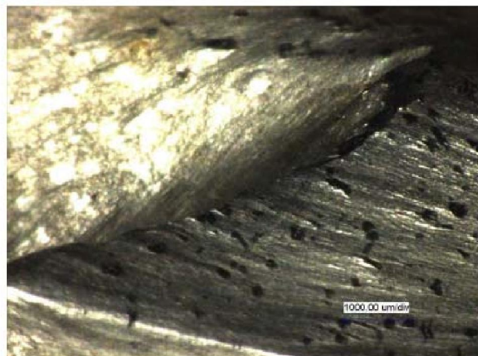
Figure 3: A directional groove and dark spots on the liner of a slurry pump (x200).
