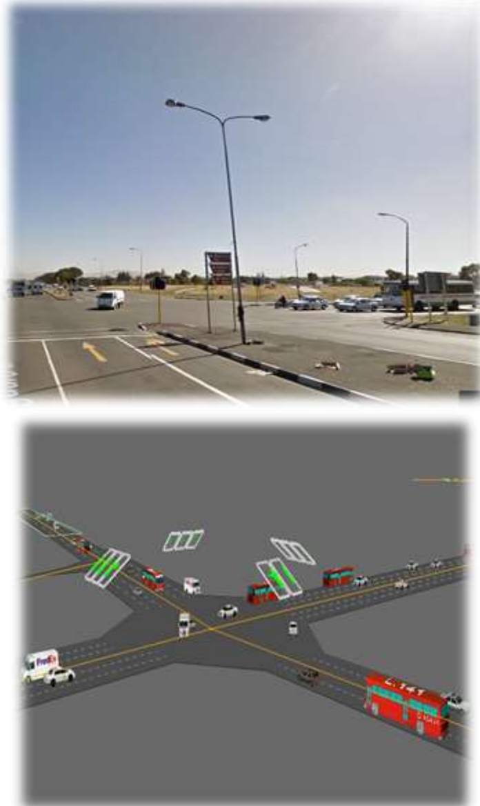
Figure 2-2 a screenshot of an intersection geometry as coded into the model
