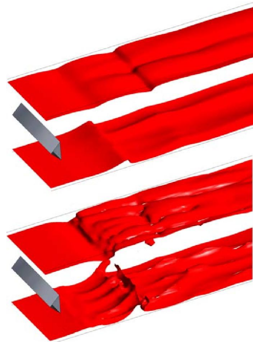
Figure 7 \theta=0.5 isosurfaces at a time-step, for Re=2,500 , top: 3D URANS, bottom: LES.
