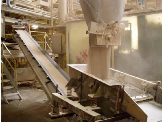
Figure 4: Spray dryer outlet and conveyor belt inlet.
