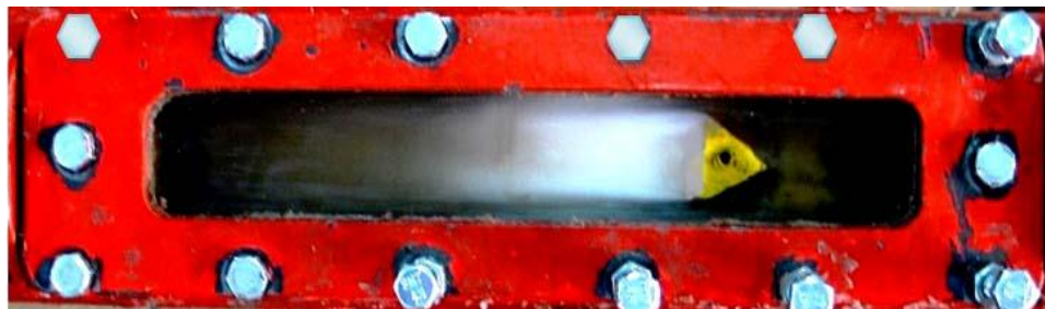
(c) Increasing of developed cavitation at ( p_o = 155 kPa Q = 4.77 lit/sec )
