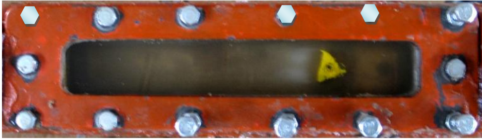
(a) Starting of cavitation inception ( Q = 3.9 lit/sec )
