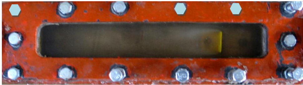
(a) Starting of cavitation inception ( V= 2.5 m/sec Q = 2 lit/sec )
