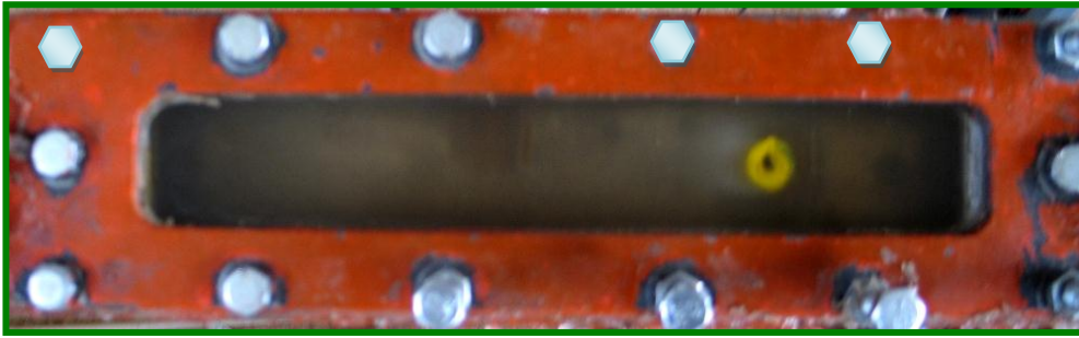
(a) Starting of cavitation inception ( Q = 4.95 lit/sec )
