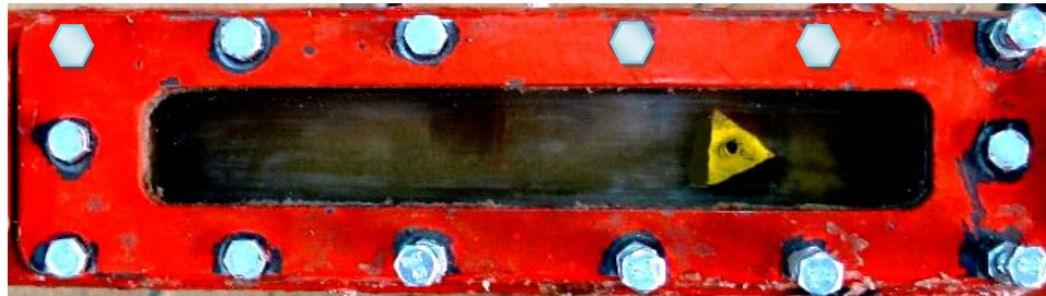
(a) Starting of cavitation inception ( Q = 2.91 lit/sec )
