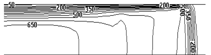
Figure 3 Axial velocity distribution (Case A) at t=1 \times 10^{-5} s
