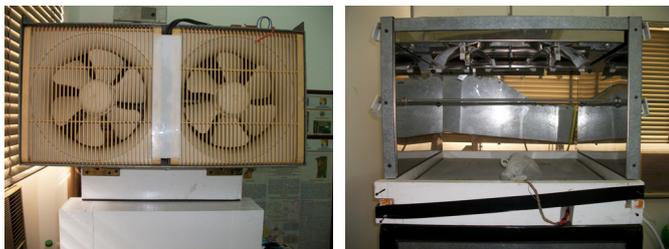
Figure 9 Test-Rig Supply Fan Section and Lighting Fixtures Over Slab For Simulating Wind Speed & Solar Radiation
