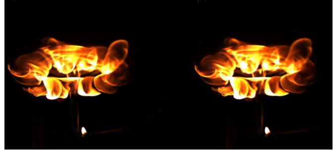
Fig. 4 Stereo image pair of the flame at 250 ms after ignition
