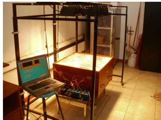
Figure 6 Experimental arrangement: Solar simulator, solar cooker and acquisition device
