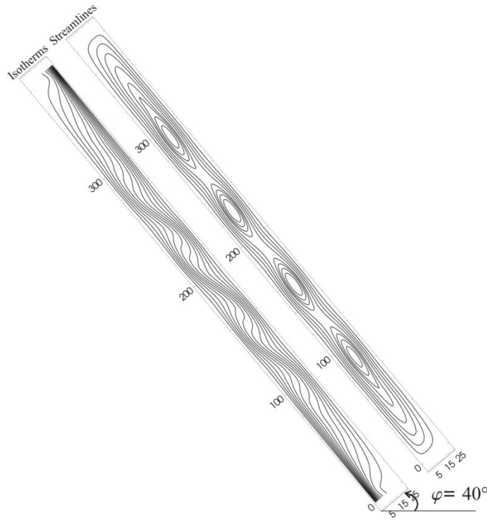
Figure 2 Isotherms and streamlines for A=16 and \varphi = 40^\circ
