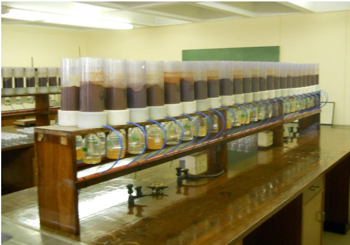
Figure 4.2 Example of leaching columns used
