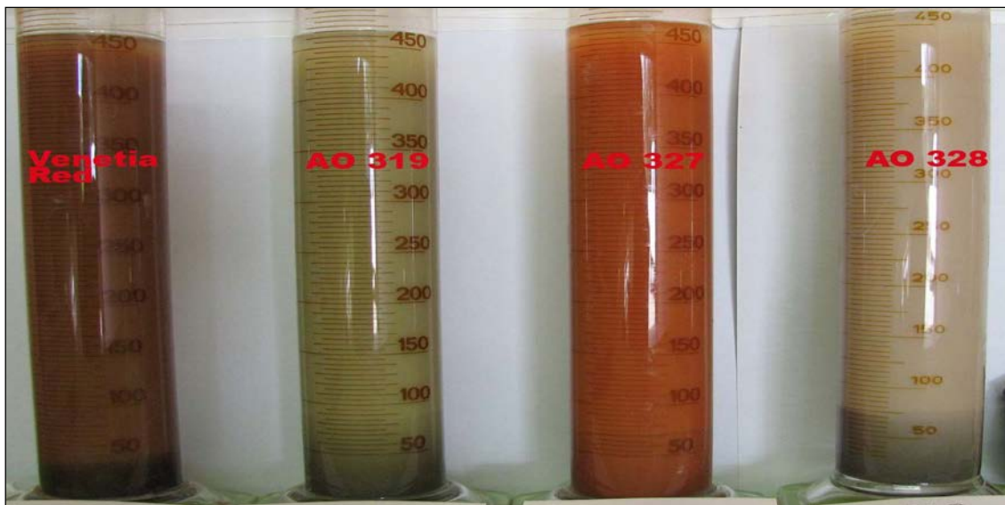
Figure 39: Natural settling of Venetia Red, AO 319, AO 327 and AO 328 after 60 minutes.
