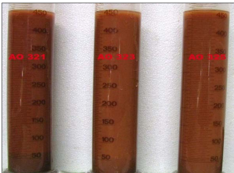
Figure 41: Natural settling of AO 321, AO 323 and AO 325 after 60 minutes.
