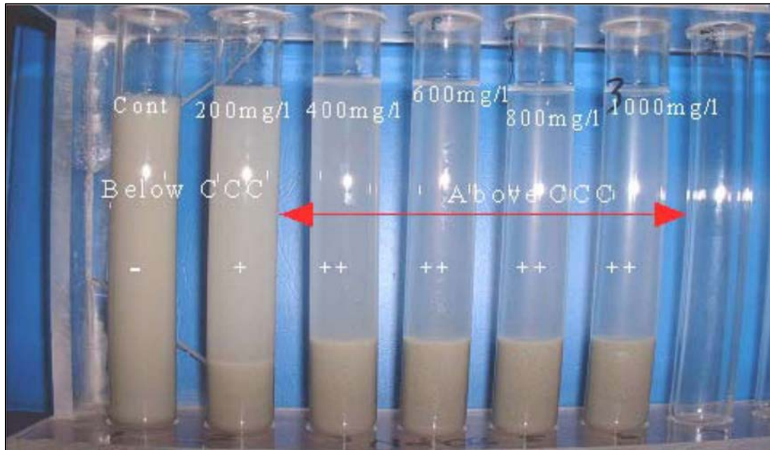
Figure 22: Example of coagulant test (Vietti & Dunn 2003).
