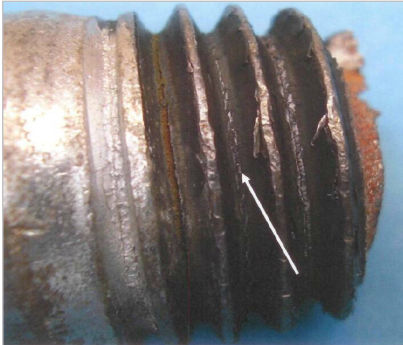
Figure 5.16: – Bolt specimen, cracks shown in thread roots (17).
