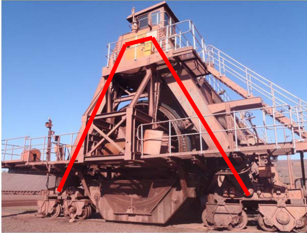
Figure 3.13: Side view of drum reclaimer, fixed legs highlighted.
