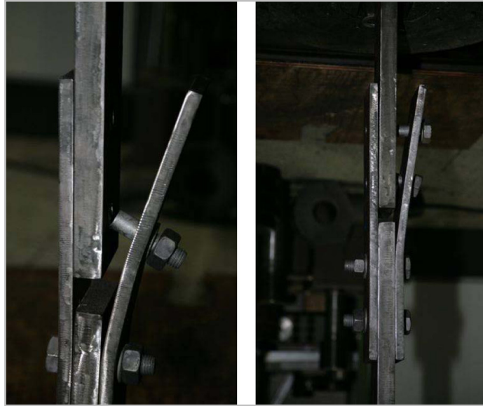
Figure 5.14: Typical 4-bolted connections after the tensile test (19).
