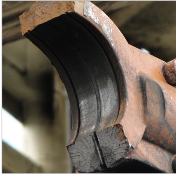
Figure 5.9: Cylinder clevis fracture plane, lubrication channel noticeable.
