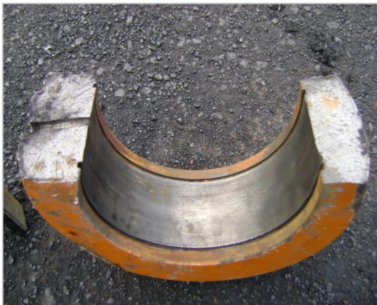
Figure 5.4: Failed cylinder clevis half.
