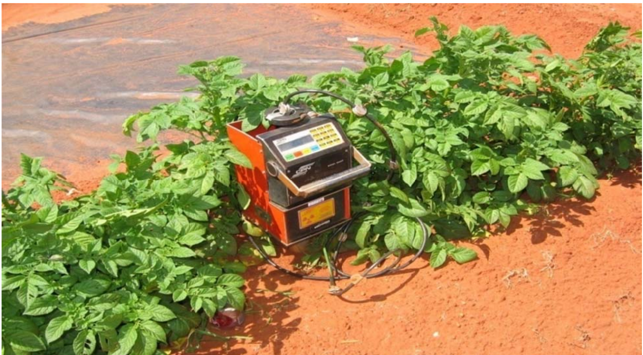
Figure 13: Soil water content measurement with a neutron probe on the ridge of a 3:1P plot during the 2009/2010 potato growing season.
