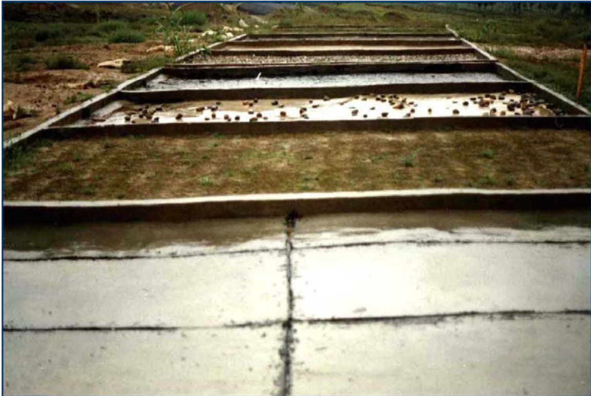
Figure 2.6: A photograph of an experimental plot layout showing different surface treatments with the concrete plot in the front, followed by a natural loess slope, gravel covered plastic film, and other treatments ( Li et al. , 2004).
