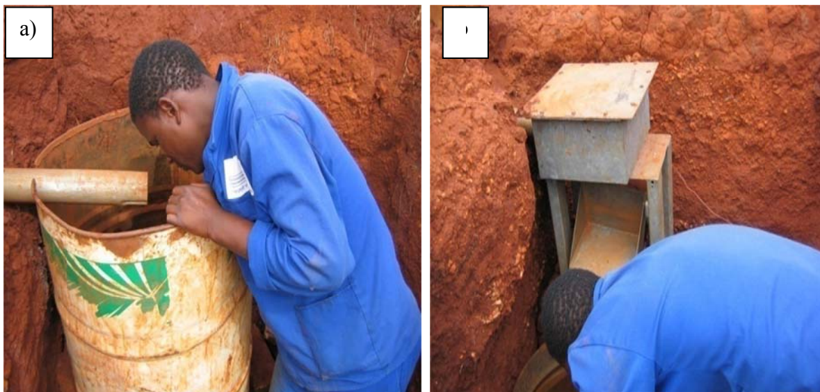
Figure 5.2: Runoff and sediment collection 1: a) adjusting the 200-L drum and b) collection of runoff and sediment from a 100-L drum under a tipping bucket.
