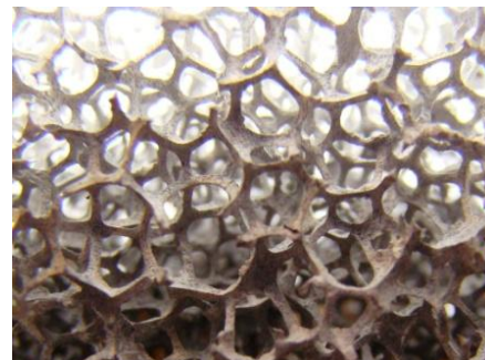
Figure 1 Illustration of the complex shapes in 10 PPI metal foam (in-house manufactured)
