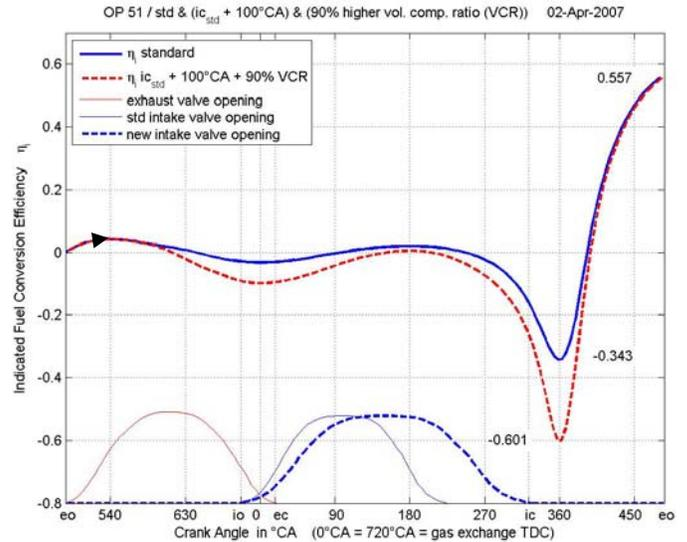
**Figure 9** (indicated fuel conversion) Efficiency–Crank Angle diagram (SV & 2V)
