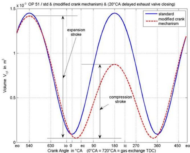
Figure 10 Volume-Crank Angle diagram (SV & 3V)
