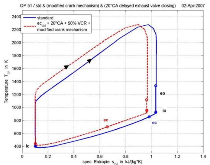
Figure 12 Temperature-(specific) Entropy diagram (SV & 3V)
