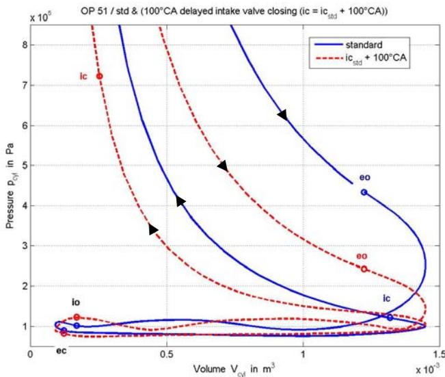
Figure 4 Pressure-Volume diagram (SV & 1V)
