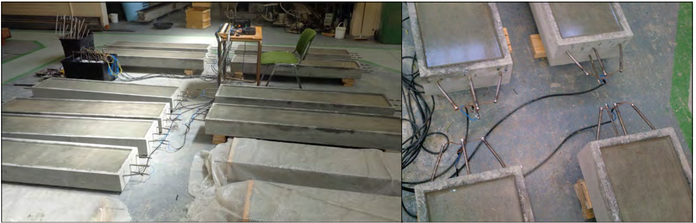
Figure 4 Accelerated corrosion setup of slab specimens
