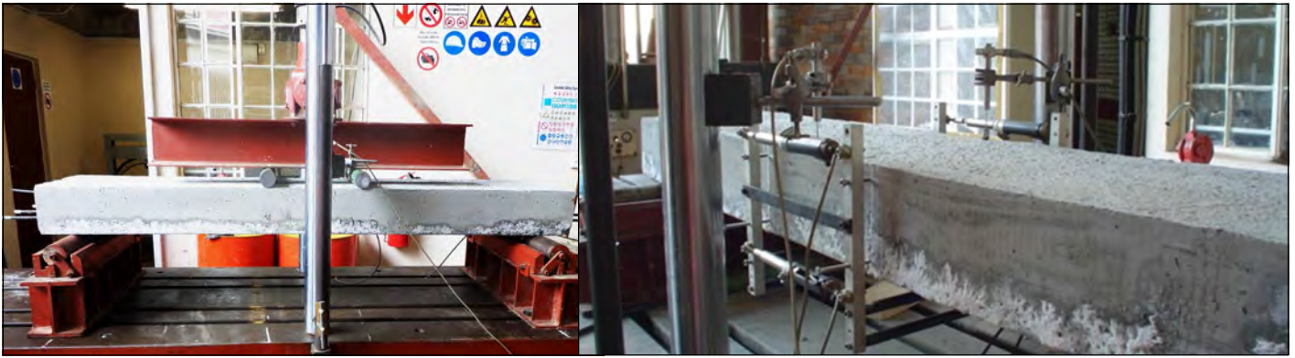
Figure 6 Testing of slabs
