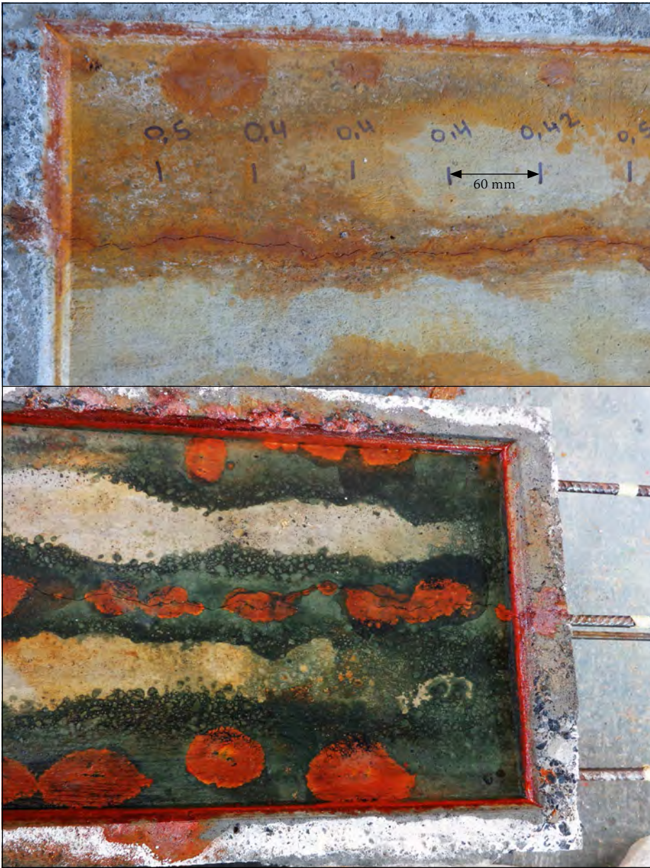
Figure 9 Longitudinal crack along the middle of the slab
