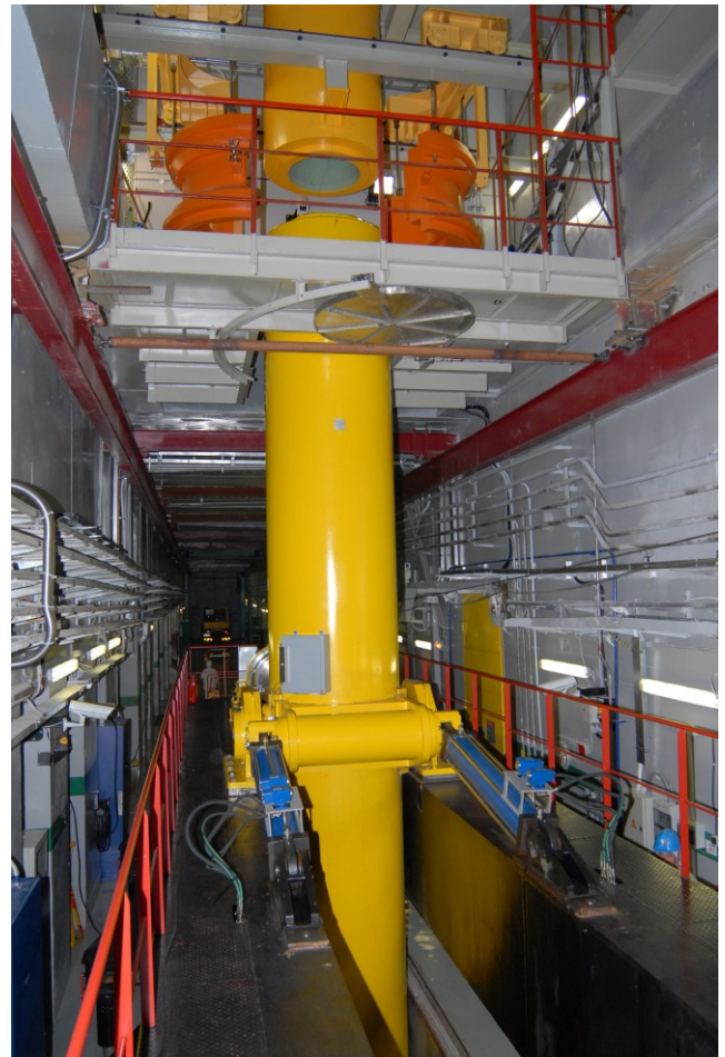
Figure 1 Container for SFAs in vertical position for fuel loading
