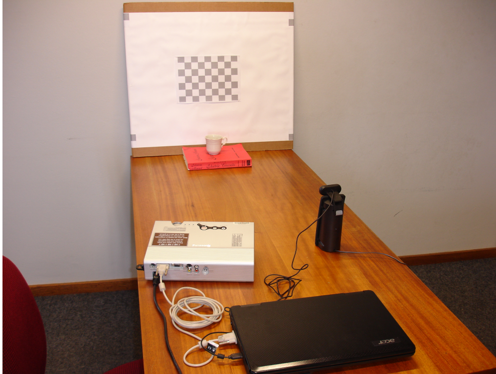
Figure 5.13: Experimental structured light setup.
