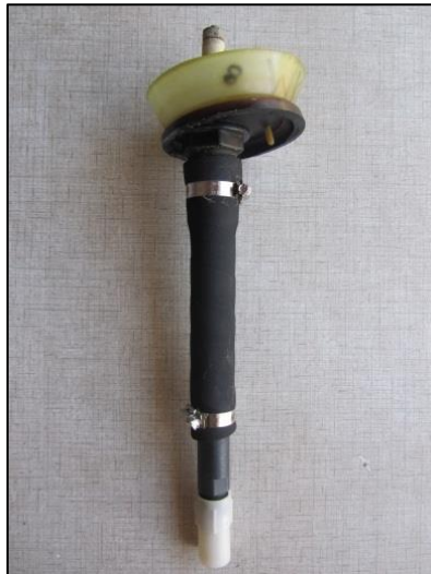
Figure 5.1 Indwelling pH logging system used to measure ruminal pH in 10 minute intervals prior insertion into the rumen
