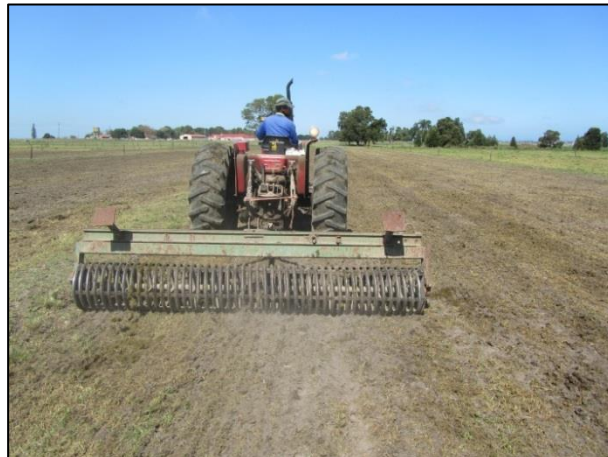
Figure 3.4 The 2.33 m Cambridge type light land roller
