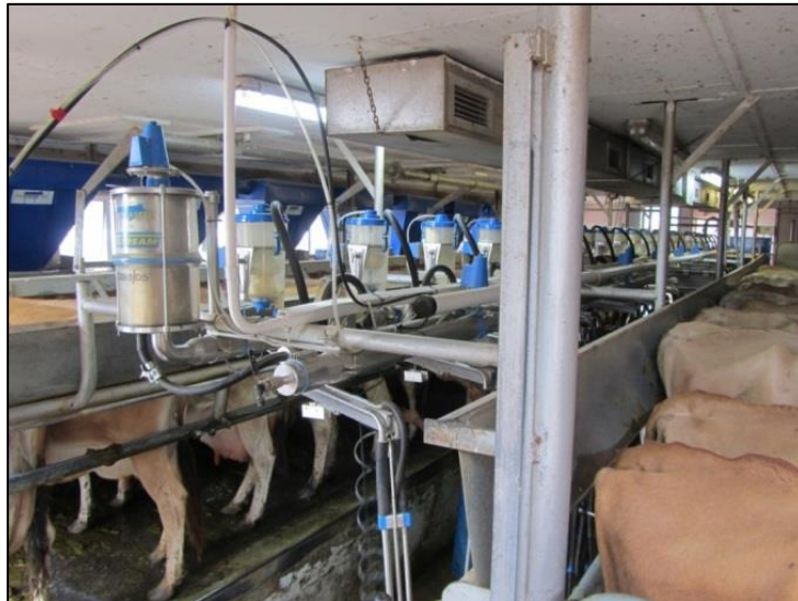
Figure 4.2 Twenty-point Dairy Master swing over milking parlour with weigh-all electronic milk meters used during the study to obtain milk data
