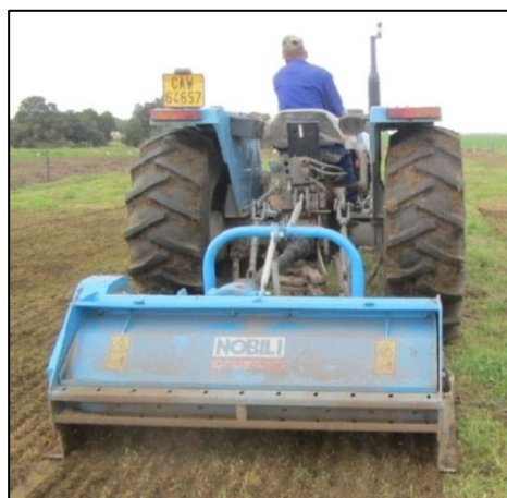
Figure 3.2 The 1.6 m Nobili mulcher with 24 blades
