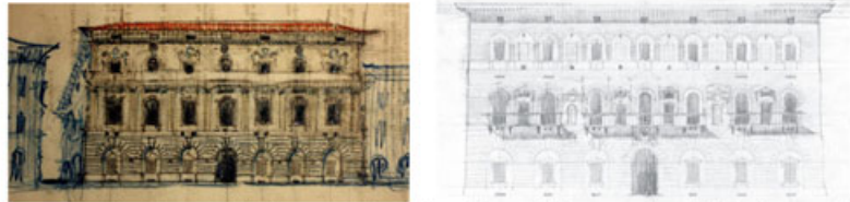
Above: From the Eaton Collection - study drawings Eaton did as a student (dating from c. 1927) of Italian Renaissance palace facades, with their typical tripartite division and underlying classical proportions and positions of principal elements. Below is a meticulous study drawing that he had done of the garden screen at the Italian Renaissance Palazzo Bernardi, Micheletti, Lucca, Italy (early 1500s) (Eaton Collection, UP Repository).
