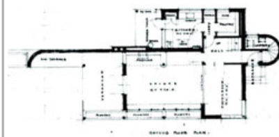
Similar to the Tugendhat House (1930), Brno by Van der Rohe; and the layered, compartmentalized planning of Wright's Robie House (1909), the service block slides behind the main living volume. The free plan is reserved solely for the living volume.
