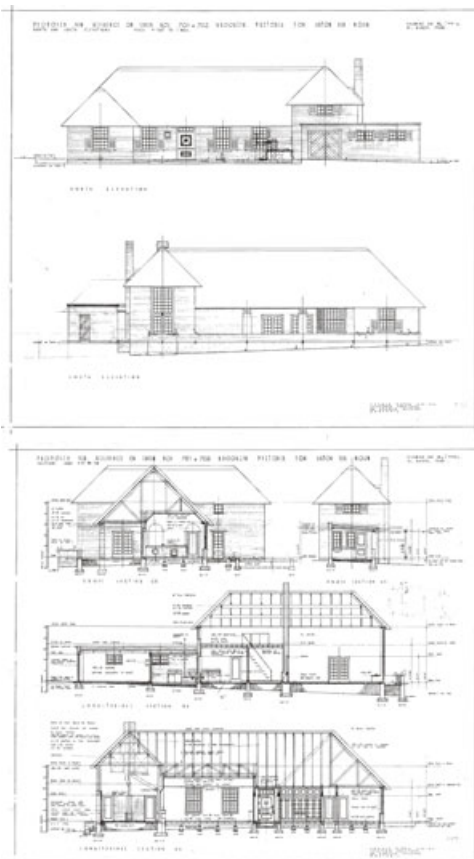
Figure 56 (top): The letter-type plan for House and Studio Van Wouw (1937–1938). The house is currently owned by the University of Pretoria and is in pristine condition. Figure 57 (left): Sections and elevations of House and Studio Van Wouw* , Corner of Rupert and Clark Streets, Brooklyn (1937–1938). Figure 58 (above, detail): Section of House and Studio Van Wouw* , Corner of Rupert and Clark Streets, Brooklyn (1937–1938).
