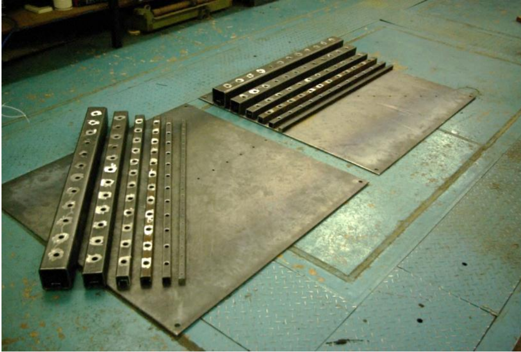
Figure 3-15 Cleats used during the dynamic cleat test
