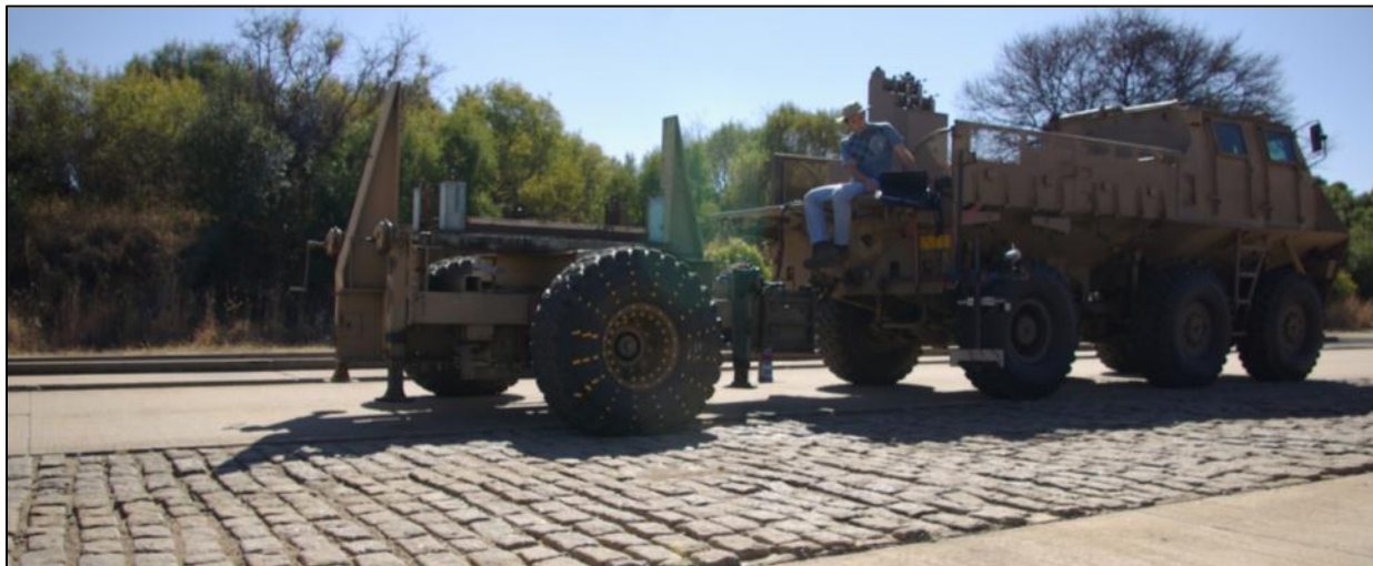
Figure 3-25 Belgium paving validation test
